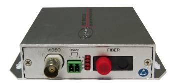
The One Channel Analog Video, and 2 bidirectional channel reverse Audio of our products, use advanced analog and digital technologies for pursuing high performance bidirectional data transmission over fiber optic. The transceiver can send signals more than 100 kilometers on fiber.
